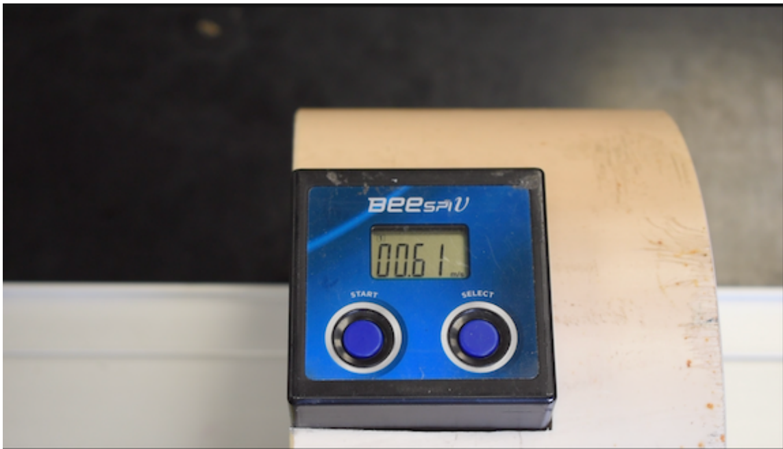
Figure 2. Photogate (velocity sensor reading 0.61 m/s)
